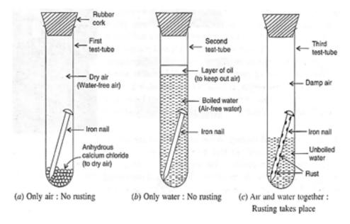
In the first test-tube containing iron nail, we put some anhydrous calcium chloride and close its mouth with a tight cork. Anhydrous calcium chloride absorbs water moisture from the damp air present in the test-tube and make it dry. In this way, the iron nail in the first test-tube is kept in dry air (having no water vapour in it).
