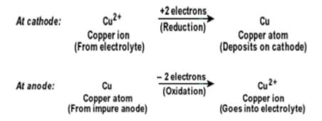
Pure copper is scraped or removed from the cathode. Anode becomes thinner as the electrolysis process proceeds. Some important metals like gold and silver are present in the anode mud. These can be recovered separately.
